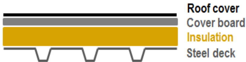
Figure 9 - Placement of cover board in a roof assembly (Image source: Rich Gallagher, Zurich)
