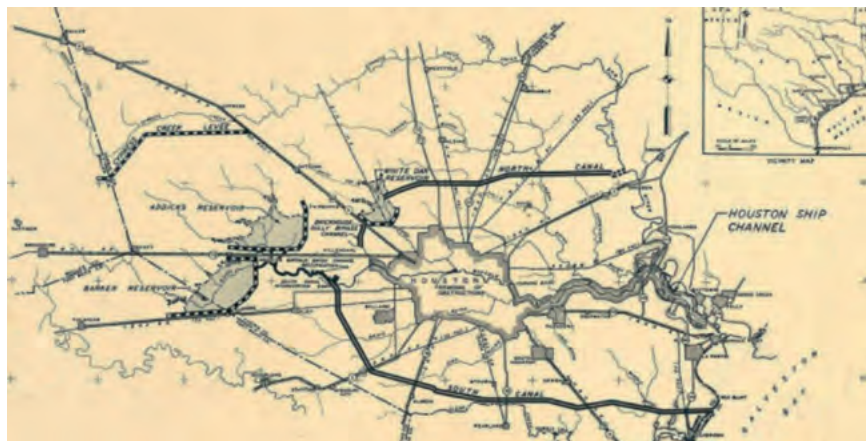
Figure 5: Original 1940 Flood Control Plan for Houston, showing Addicks and Barker Reservoirs to the west, the Cypress Creek levee to the west-northwest, White Oak Reservoir to the northwest, and North and South Canals circling the city and emptying into Galveston Bay to the east. (Source: USACE, 1940).
